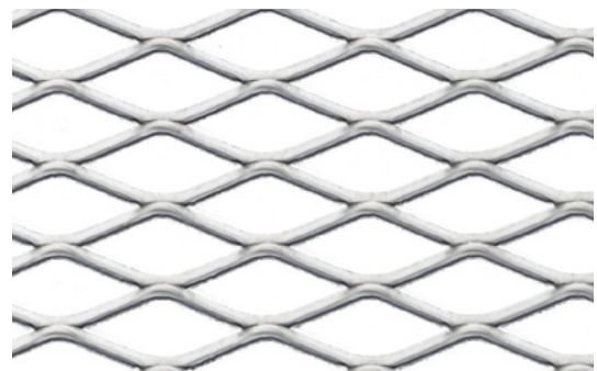
Masche 30 x 12 x 2,0 x 1,5 [mm] Mesh freier Querschnitt ca. 66,7% free cross-section approx.
