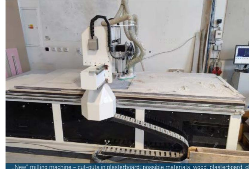
„New“ milling machine – cut-outs in plasterboard; possible materials: wood, plasterboard, chipboard, Fermacell, etc.
