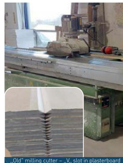
„Old“ milling cutter – „V, slot in plasterboard
